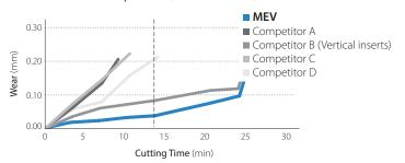
$Cutting\ conditions: Vc = 180\ m/min, ap \times ae = 3 \times 10\ mm, fz = 0.1\ mm/t, \varnothing 20, dry, workpiece: X153CrMoV12\ (30 \sim 35HS)$
