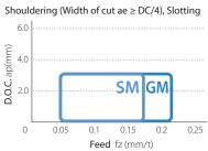
Cutting conditions: Vc = 150 m/min, ae = DC mm, Workpiece: C50
