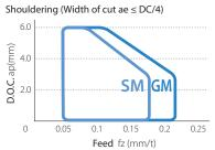
Cutting conditions: Vc = 150 m/min, ae = DC/4 mm, Workpiece: C50
