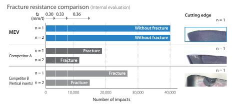
Cutting conditions: Vc = 120 m/min, ap  $\times$  ae =  $2 \times 10 \text{ mm}$ , fz = 0.3 - 0.36 mm/t,  $\emptyset = 20 \times 10 \text{ m/s}$  Workpiece: 42 CrMo4 ( $37 \sim 39 \text{ HS}$ )
