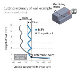
Cutting conditions : Vc = 200 m/min, ap  $\times$  ae=3  $\times$  10mm (4 pass), fz = 0.15 mm/t,  $\phi$ 50 (5 inserts), Dry Workpiece : C50
