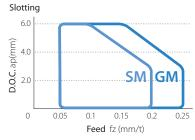
Cutting conditions : Vc = 150 m/min, ae = DC mm, Workpiece : C50
