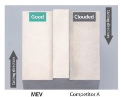
Cutting conditions : Vc = 180 m/min, ap  $\times$  ae=3  $\times$  40mm, fz = 0.1 mm/t,  $\emptyset$ 50 (5 inserts), Dry Workpiece : C50
