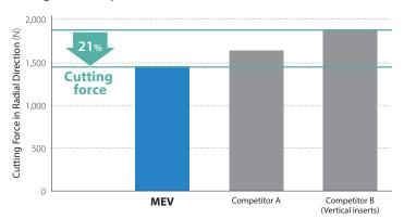
$Cutting\ conditions: Vc = 200\ m/min, ap \times ae = 3 \times 18\ mm, fz = 0.10\ mm/t, \varnothing 20\ (3\ inserts), Dry\ Workpiece: 42rMo4$
