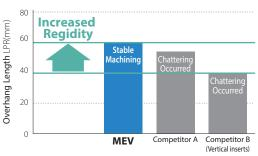
$Cutting\ conditions: Vc = 200\ m/min, ap \times ae = 3 \times 18\ mm, fz = 0.10\ mm/t,\ \varnothing 20\ (3\ inserts), Dry\ Workpiece: 42CrMo4$
