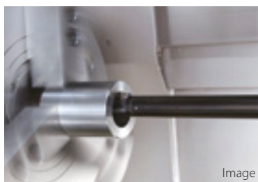
KAV-G20-10D / KAVH20-SCLCR09 CCMT09T304PP Overhang length: 140 mm (7D) / 200 mm (10D) Workpiece: SCM435
